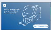
Close the drawer and press "Start Measurement" once your incubation time has finished. The reader will measure the test cassette (N2).
