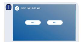
On the SKIP INCUBATION screen, press "YES". if the incubation time is controlled via an external timer. Press "NO" if the incubation time should be counted down by the reader.
