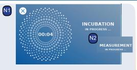
The reader will now run the test, starting with the test-specific incubation (N1), followed by test cassette measurement (N2).
