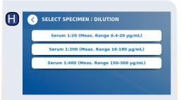
Some test methods may require a selection of the specimen type and/or the sample dilution.
