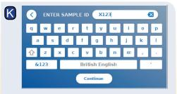
Enter patient/sample ID either via the keyboard, or via an external barcode scanner\*
