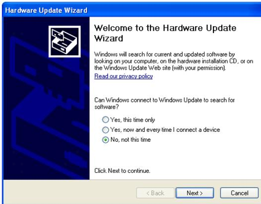
Immediately after the installation of the USB device driver the installation of the virtual COM Port will be initiated. Select the last button “No, not this time” and press “Next”.
